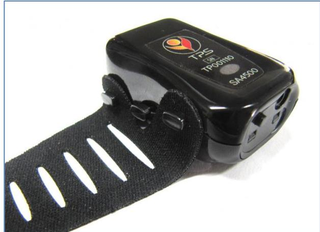
2. Apply the eVu TPS to your finger, with the writing on the label oriented upward and with the "On" button pointing toward your hand. You can try using the eVu TPS on any finger, but the index and middle fingers are recommended for best results. The device should be placed near the end of your finger. The two metal plates on the underside of the sensor should be resting against your skin, for best results, against fleshy parts of the finger.
