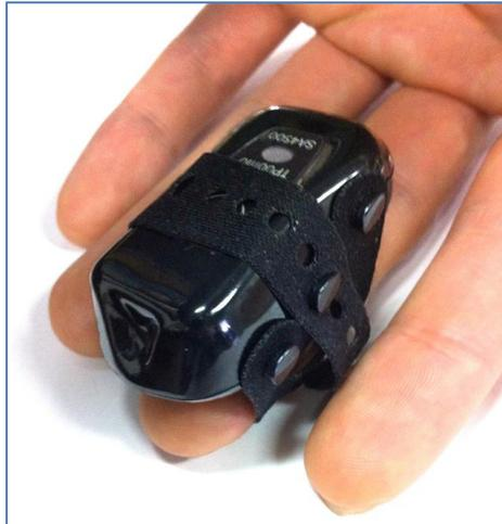
When properly fastened, the fabric strap will cover the eVu TPS logo, but the indicator light will be visible when the device is on.
