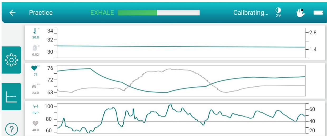
Signal View presents three-line graphs representing the live signal for temperature and skin conductance, respiration and heart rate, and raw pulse signal and heart rate variability. Labels for each modality are shown on the top and bottom left of the graphs canvases along with your current values.
